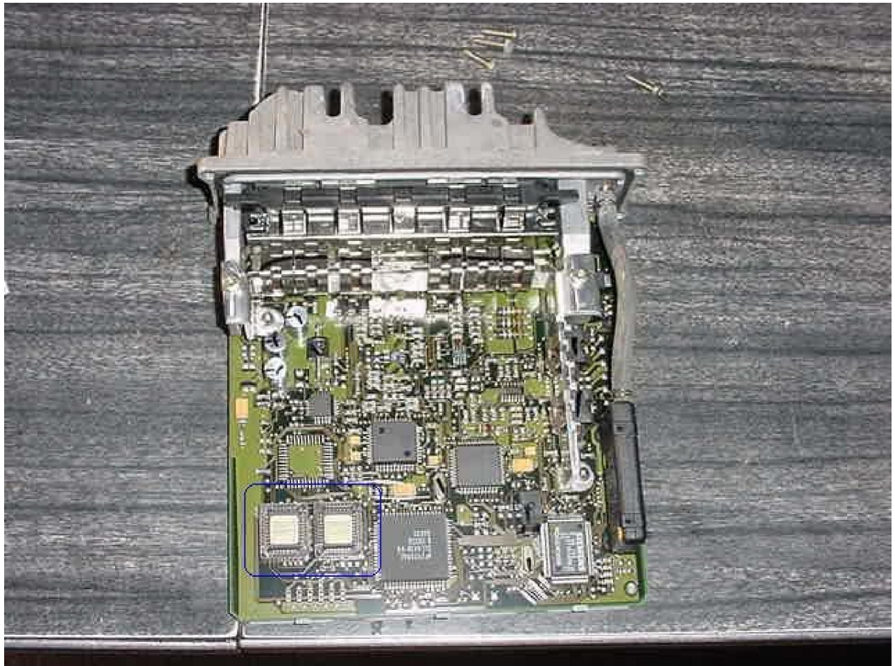
Here's a snap shot of the inside of the ECU. The chips of interest are in the lower left hand corner.
