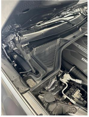
B. Remove this by pulling the weather stripping up and one clip on the lower corner
