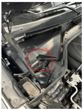
C. Remove the cabin air filter by releasing the one clip in the middle and pulling up.
