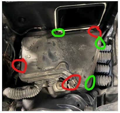
F. Slide the white locking clip towards the front of the car inorder to unlock.
