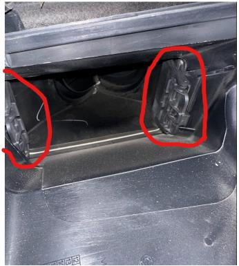
E. Once removed you will get access to the ECU cover. By removing the 3 metal clips (red) and 3 push tabs (Green)
