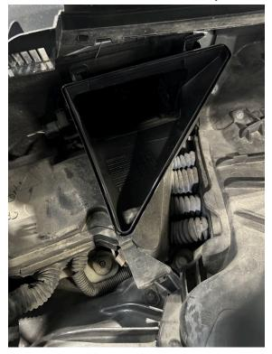
D. Inside the cabin air filter duct will be 2 grab clips that you will need to remove almost like a shop vacuum
