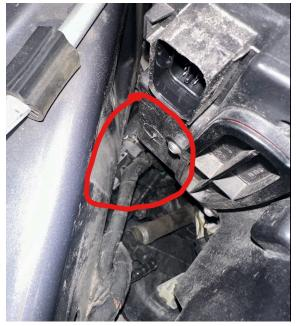
C. The SCR is in a "cage" open the cage and wiggle the SCR out.
