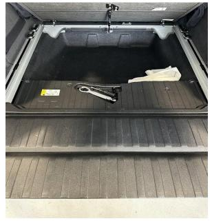
C. Once removed please disconnect the negative from the main battery.(10mm socket)
