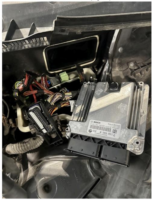
H. Under the nest of wires is the ECU, unplug and pull the ECU out.
